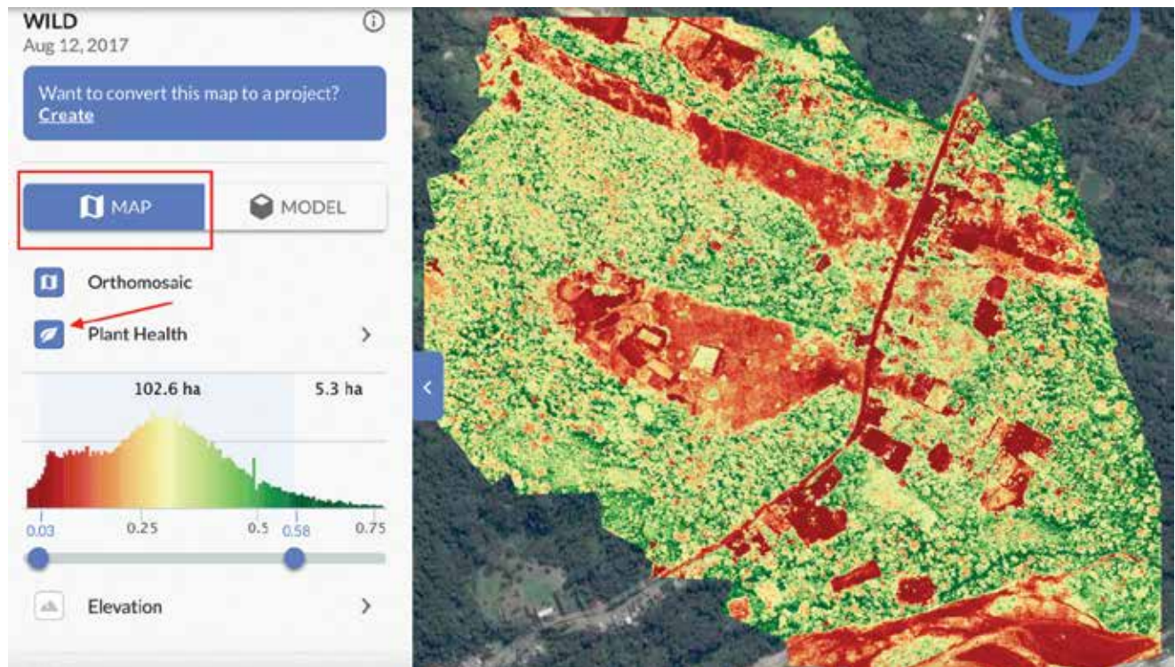
Figure 3.14. UAS thermal and multispectral imagery of city trees showing their relative health (Ric Stephens; website screen capture courtesy of DroneDeploy)
