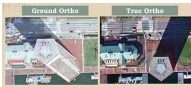
Figure 3.4. An uncorrected orthophoto (left) shows perspective distortions; a rectified orthophoto (right) flattens and scales the entire image. (Penn State University, OPEN.ED@PSU)
